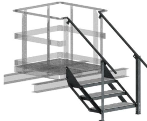
Stairs allow for 5" - 7" vertical adjustment per step
