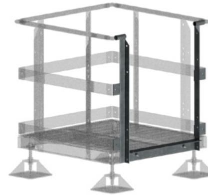
MOPEN-4 must be used for handrail attachment
