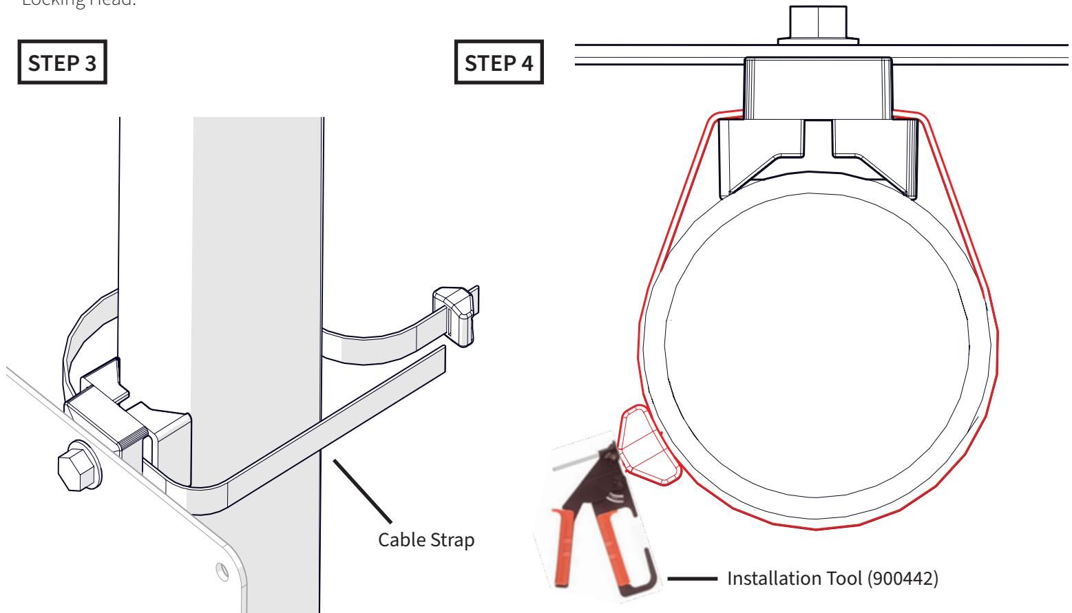
**STEP 4:** Use Cable Strap installation tool (900442 or equivalent) to tighten **Cable Straps** and flush-cut tail to Locking Head.
