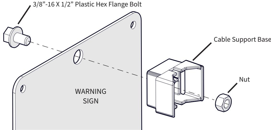
**STEP 3:** Pass one **PIM Shield Cable Strap** through each **Support Base**, around pipe or angle member, and back through Locking Head.
