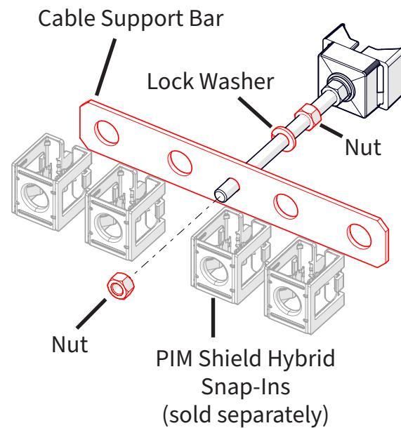
**STEP 2:** Install Cable Support Bar with hardware as shown (Torque hardware to 10 Ft-lb, ConcealFab Tool PN: 900053)
