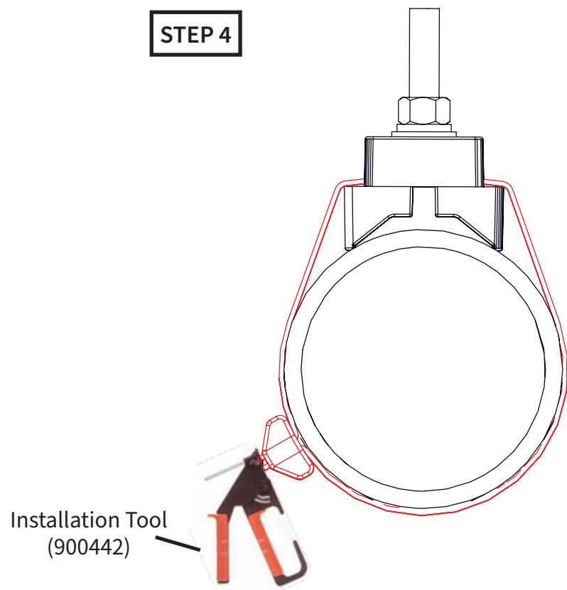
**STEP 4:** Use Cable Strap installation tool (900442 or equivalent) to tighten Cable Strap in position shown and flush-cut tail to Locking Head.
