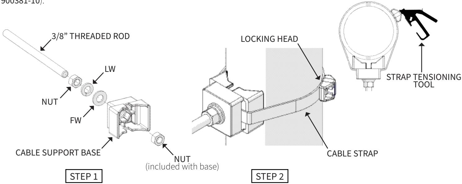
**STEP 2:** Secure Snap-in Support Base to a round or angle member using Cable Strap(s) (PN's: 900443-16-50 or 900443-27-25). Use Strap Tensioning tool (900442 or equivalent) to tighten Cable Strap(s). Trim Strap(s) flush to Locking Head.
