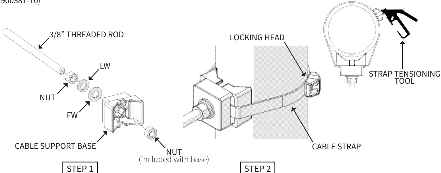
**STEP 2:** Secure Snap-in Support Base to a round or angle member using Cable Strap(s) (PN's: 900443-16-50 or 900443-27-25). Use Strap Tensioning tool (900442 or equivalent) to tighten Cable Strap(s). Trim Strap(s) flush to Locking Head.
