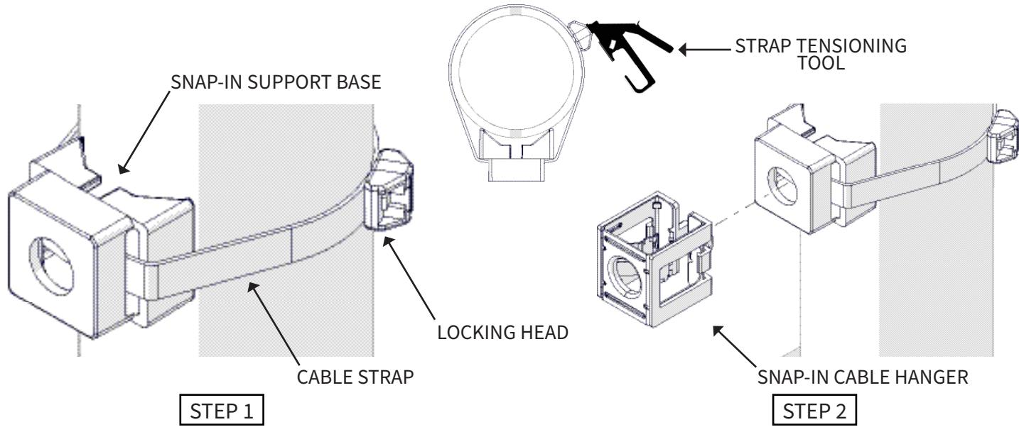
**STEP 2:** Install low PIM stackable Snap-in Cable Hangers (sold separately, PN's: PSHS-xxxx-10 or PSPS-xxx-10) as required into mounting hole provided. Maximum stack height = 3.
