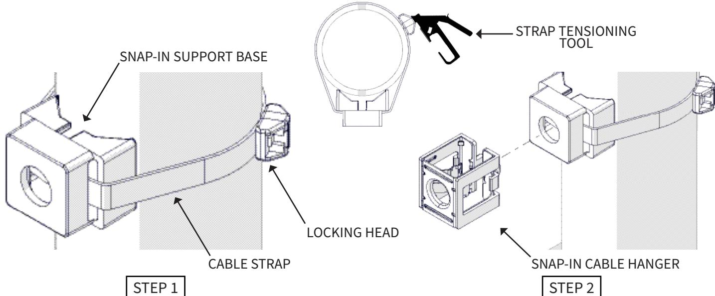
**STEP 2:** Install low PIM stackable Snap-in Cable Hangers (sold separately, PN's: PSHS-xxxx-10 or PSPS-xxx-10) as required into mounting hole provided. Maximum stack height = 3.
