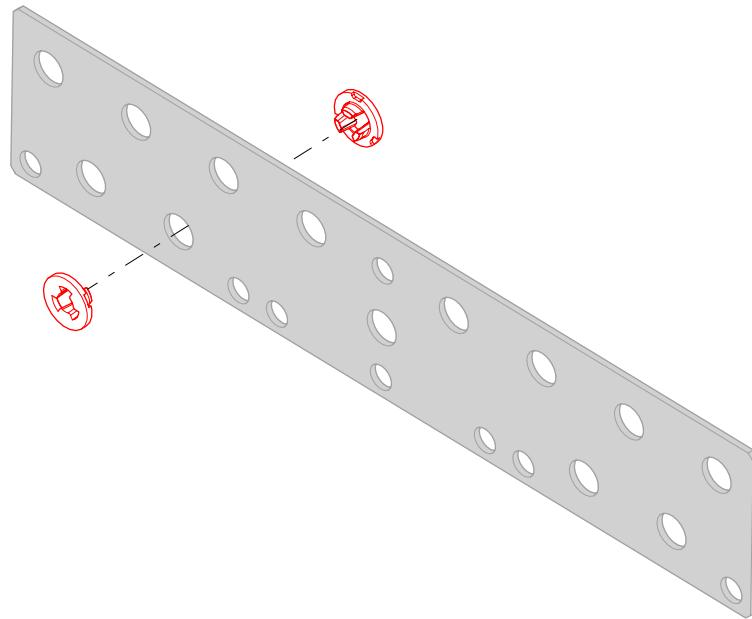
**STEP 2:** Install **threaded hardware and PIM Shield Cable Block(s)**.
