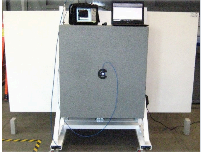
Mobile far-field millimeter-wave transmission-loss test rig for RF inspections.
