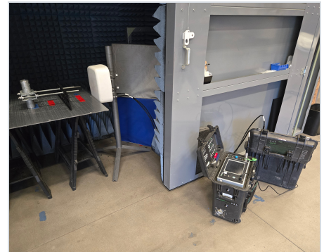
Radiated PIM test rig, IEC 62037-8, 700 and 1900 bands.
