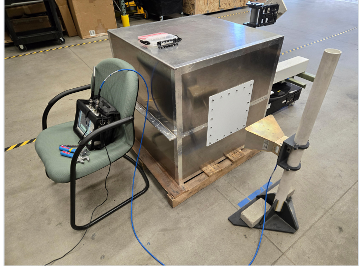
Transmission-loss test, 1–17 GHz: PIM Paint on clearWave contacting gaskets around an AI window.
