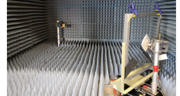
Figure 4: Antenna pattern testing, 3.6 GHz.
